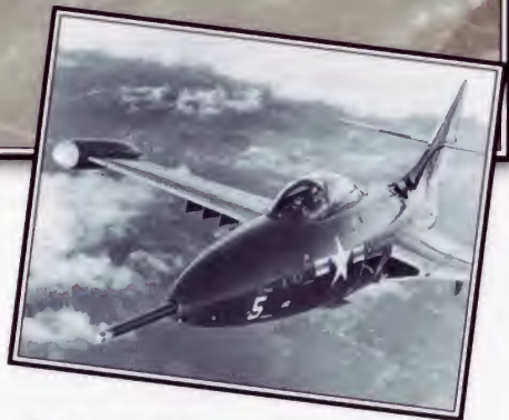
▲ The Panther gained many 'firsts' for the US Navy. It was the first USN jet to go to war, the first to use a blown flap and the first to try an inflight-refuelling system.
